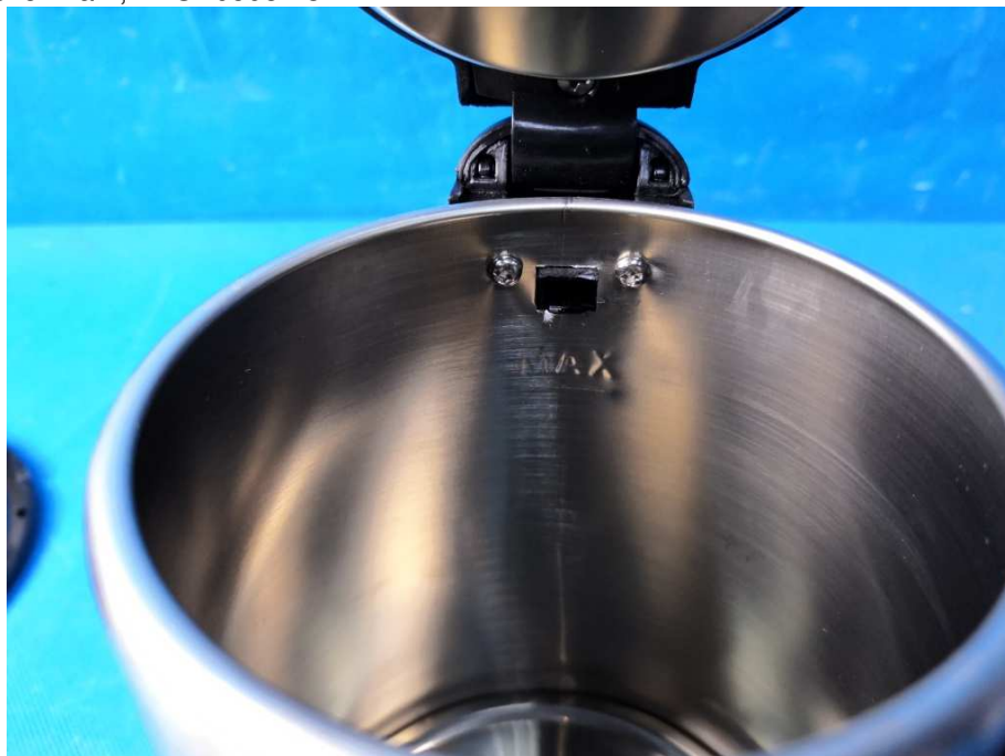
View of water level mark, TPCK0508-13
