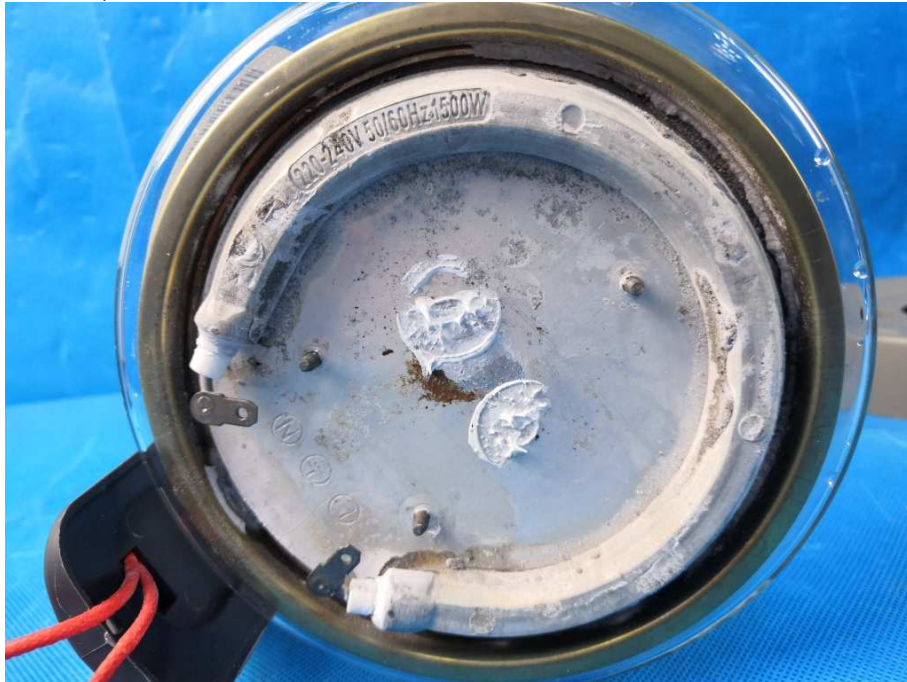
View of heating element, rated 1800 W
