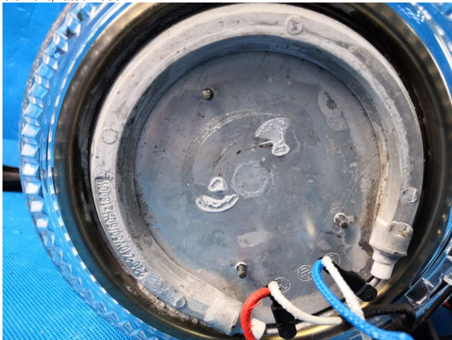
View of heating element, rated 1800 W
