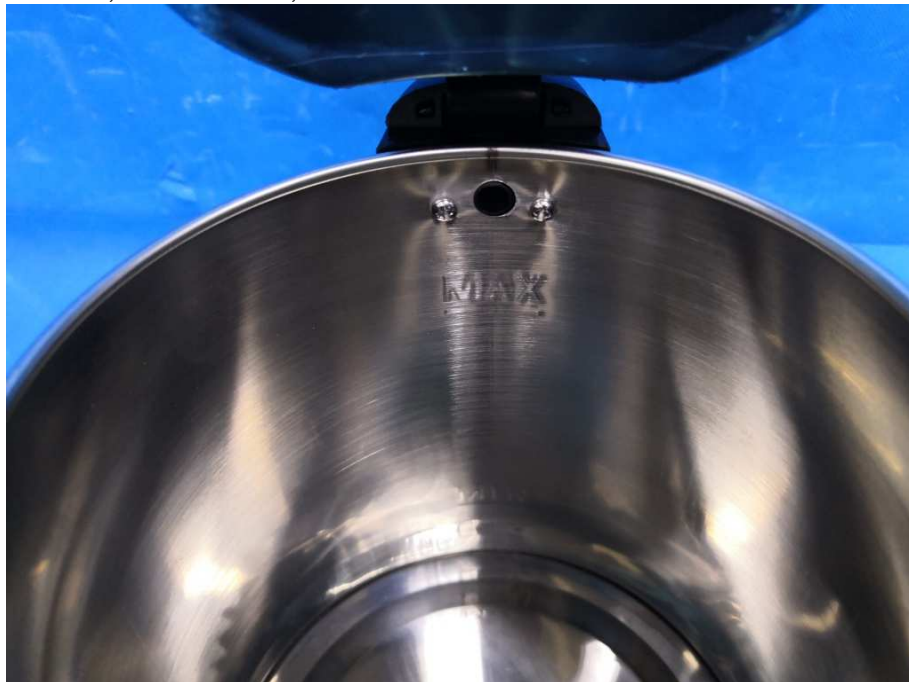
View of water level mark, TPSK8518-15, TPSK8518-18
