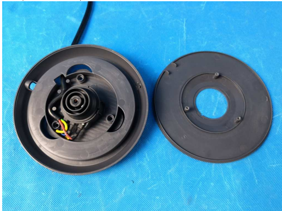
Internal view of stand, TPGK1218-15, TPGK1218-18
