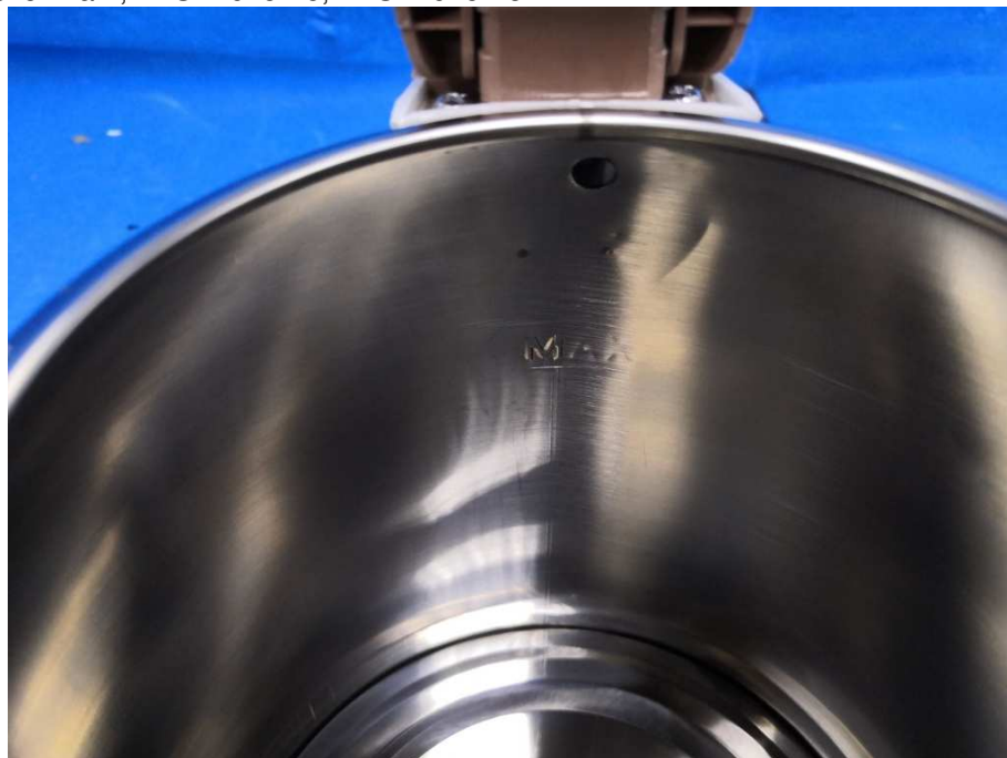
View of water level mark, TPSK7625-15, TPSK7625-18
