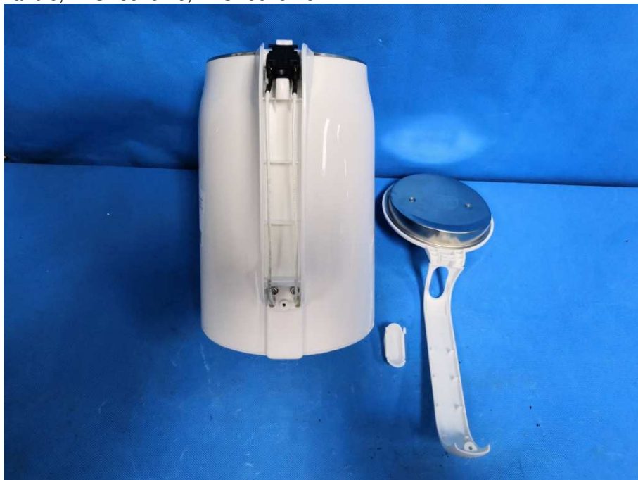
Internal view of handle, TPSK8815-15, TPSK8815-18
