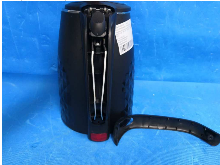
Internal view of handle, TPSK7425-15, TPSK7425-18
