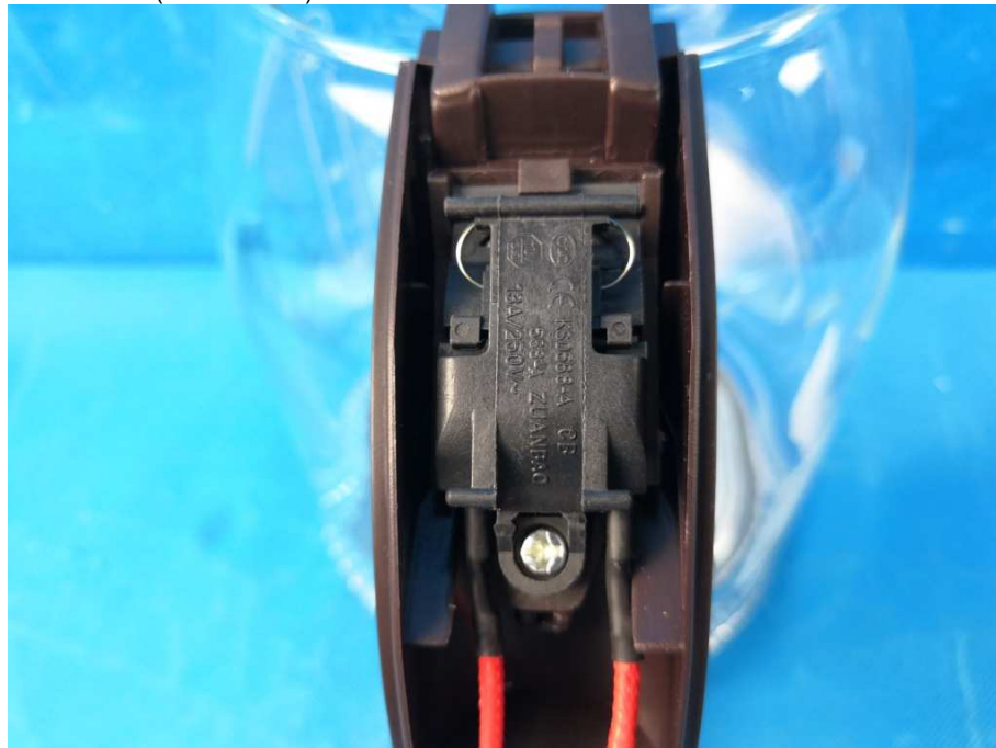
View of temperature limiter (ZUANBAO)
