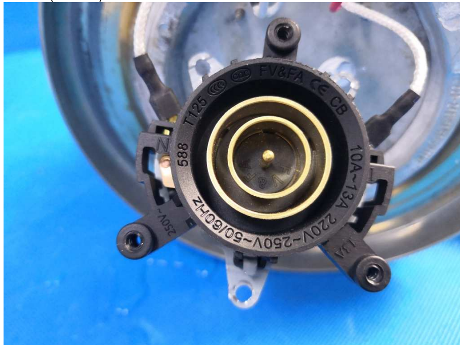
View of thermal control (FUFAN)
