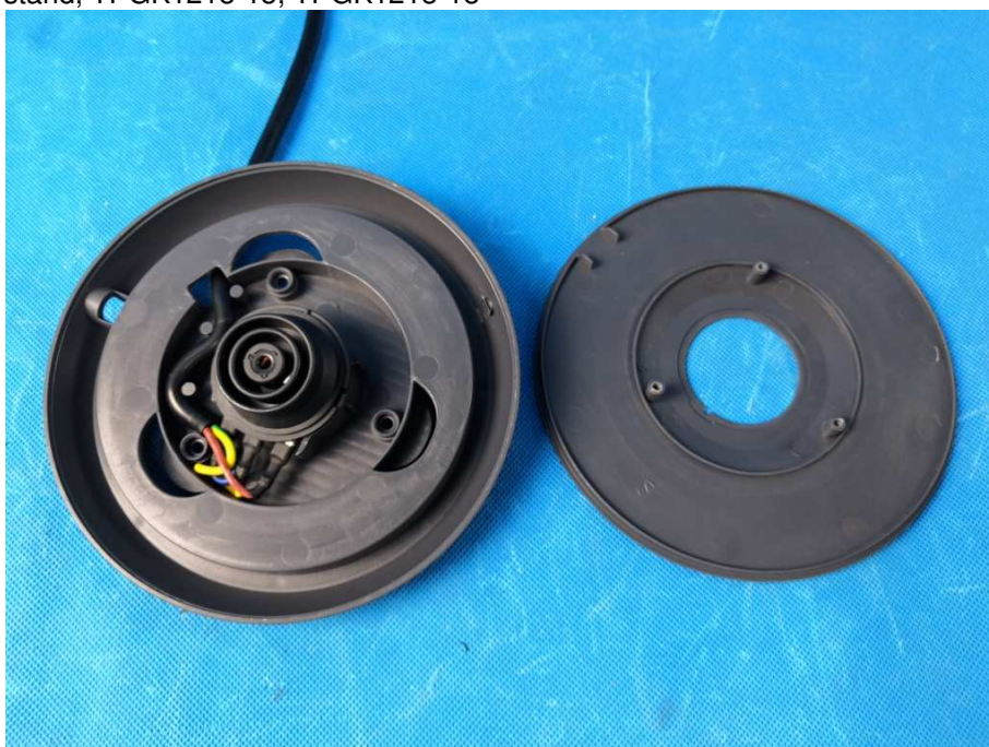
Internal view of stand, TPGK1218-15, TPGK1218-18
