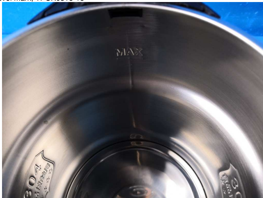
View of water level mark, TPCK0318-18
