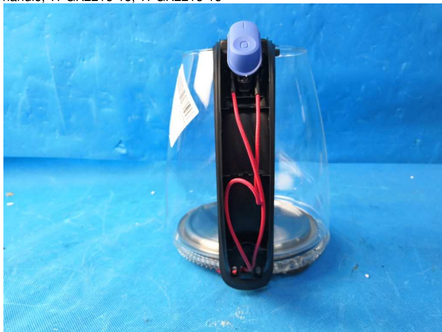
Internal view of handle, TPGK2218-15, TPGK2218-18
