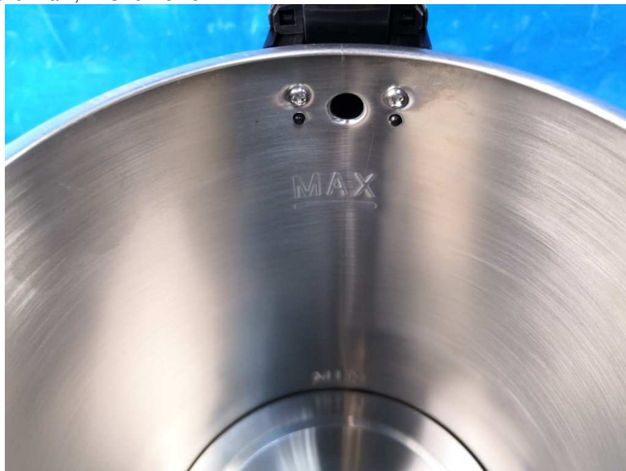
View of water level mark, TPCK0118-18
