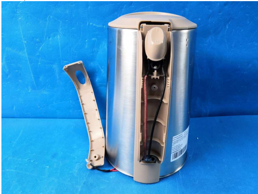
Internal view of handle, TPCK0225-18
